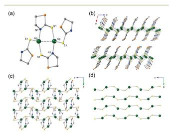
Fig. 1 Crystal structure of KGF-24. (a) Dinuclear coordination unit. Ag-Ag bond is shown by the dashed black line. (b) Packing of the 2D layer structure. (c) 2D layer structure parallel to the bc plane. (d) (-Ag-S-), network in the 2D layer structure. Color code: Ag; dark green, S1; yellow, S2; orange, N; blue, C; gray. H atoms are omitted for clarity.
