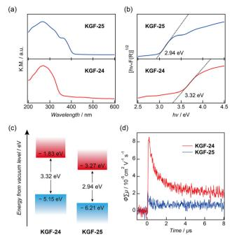
Fig. 3 Semiconductive properties of KGF-24 and KGF-25. (a) DR-UV-vis spectroscopy. (b) Tauc plot. (c) Energy diagram below vacuum level. VBM energy level was determined by PYS experiments as depicted in Fig. S7.† (d) Results of TRMC experiments ( $\lambda_{\rm ex}$  = 355 nm; red: KGF-24, blue: KGF-25).
