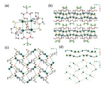
Fig. 2 Crystal structure of KGF-25. (a) Tetranuclear coordination unit. Ag-Ag bond is shown by the dashed black line. (b) Packing structure along the c-axis. (c) 2D layer structure parallel to the bc plane. F atoms are omitted for clarity. (d)  $(-Ag-S-)_n$  network in the 2D layer structure. Color code: Ag1; dark green, Ag2; teal blue, S1; yellow, S2; orange, N; blue, C; gray, O; oxygen, F; light green. H atoms are omitted for clarity.
