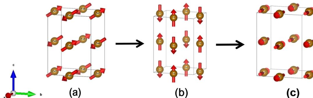
Fig. 3 Schematic representation of the DNFO91 magnetic structure at (a) 100 K:  $\Gamma_{4+3}$ , (b) 45 K:  $\Gamma_2$ , which is an incomplete metastable phase transition induced by magnetic field, and (c) 43.8 K:  $\Gamma_1$ .
