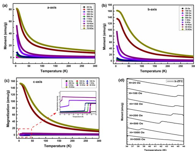
Fig. 5 The *M-T* curves of the DNFO91 single crystal measured in the ZFC mode along the (a) *a*-axis, (b) *b*-axis and (c) *c*-axis at different magnetic fields; (d) the detailed magnetization along the *b*-axis at different magnetic fields from 36 K to 45 K.
