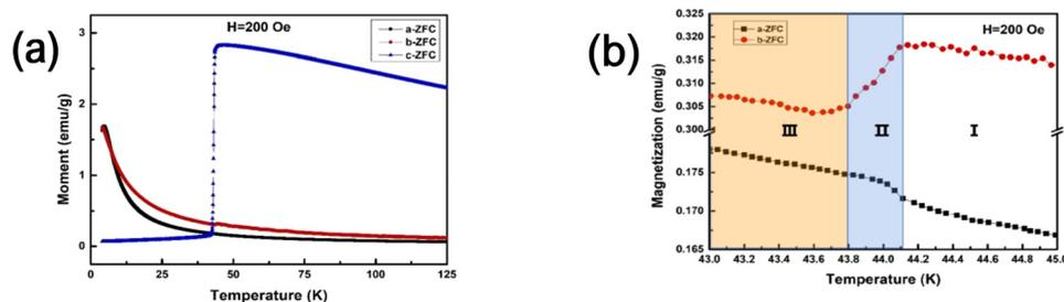
**Fig. 2** (a) The  $M$ - $T$  curves of the DNFO91 single crystal measured in ZFC mode along the  $a$ -axis,  $b$ -axis and  $c$ -axis with an applied magnetic field of 200 Oe; (b) the detailed magnetization along the  $a$ -axis and  $b$ -axis from 43 K to 45 K.
