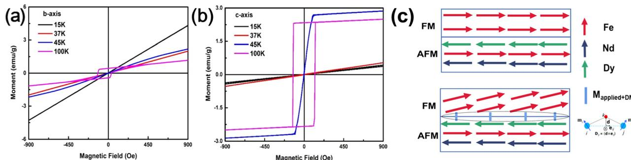
Fig. 4 The magnetization hysteresis loops at  $H_{\text{max}}$  of 1000 Oe along the (a) *b*-axis and (b) *c*-axis at different temperatures. (c) The interactions between three ions lead to an exchange-bias behavior in the DNFO91 single crystal. The arrows represent the magnetic moments of the different ions.
