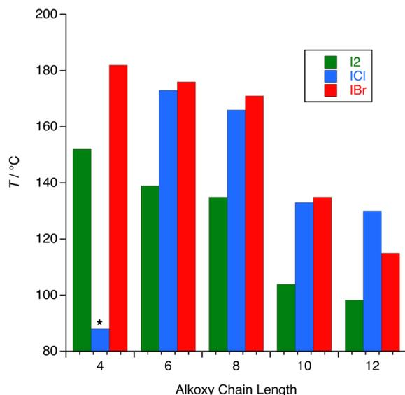
Fig. 12 Melting points of the complexes of *n*-OPhPy as a function of alkoxy chain length.
