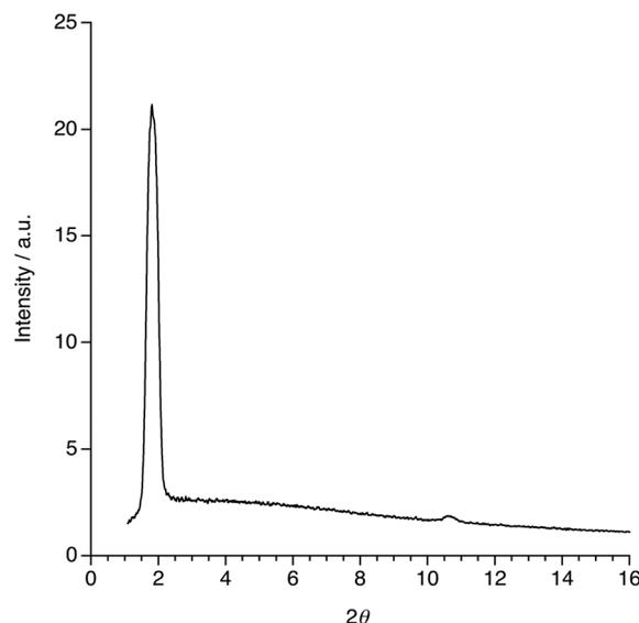
Fig. 13 SAXS data for 12-OPhPy...IBr in the SmA phase at 120 °C.
