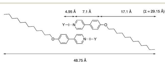
**Fig. 16** Sketch to show maximum extent of likely overlap of the halogen-bonded liquid crystals, with distances based on the structures of 4-OPhPy⋯IBr and of [12-OPhPyH]<sup>+</sup> Br<sup>–</sup>.
