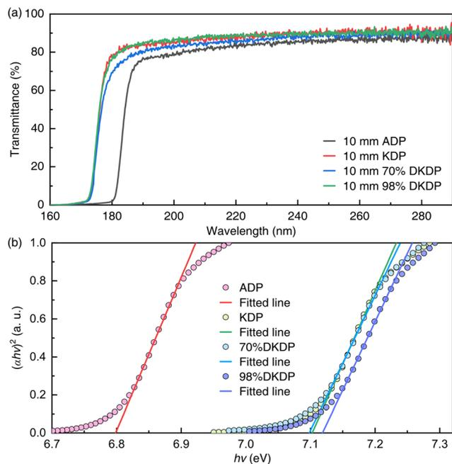
**Fig. 2** (a) Experimentally measured absolute transmittance spectra of the ADP, KDP, 70% deuterated KDP, and DKDP crystal samples in the UV spectral region of 160–290 nm. (b) Band-gap energies of the ADP, KDP, 70% deuterated KDP, and DKDP crystal samples were determined from the Tauc plots. The fitted linear parts are used to evaluate the band-gap energy at the x-axis intercept.
