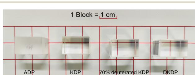
Fig. 1 Photograph of ADP, KDP, 70% deuterated KDP, and DKDP crystal samples.
