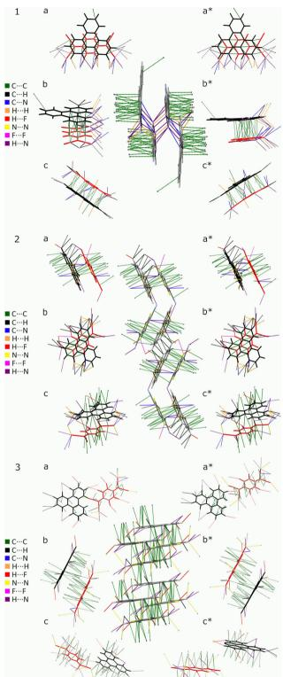
Fig. 5 Triphenylene–TCNQF $_n$  unit cells, (1)  $F_n = 0$ , (2)  $F_n = 2$  and (3)  $F_n = 4$  with cell packing (centre) surrounded by asymmetric units of TCNQF $_n$  (red) and triphenylene (black) viewed down the a, b, c,  $a^*$ ,  $b^*$  and  $c^*$  cell axis.
