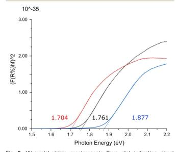
Fig. 9 Ultraviolet-visible spectroscopic Tauc plot indicating direct optical band gaps for triphenylene-TCNQ (blue), triphenylene-TCNQF2 (black) and triphenylene-TCNQF<sub>4</sub> (red).
