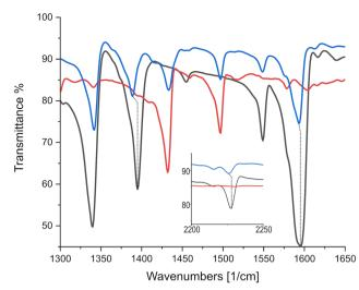
Fig. 8 IR absorption spectra identifying significant charge sensitive mode displacements between TCNQF4 and triphneylene-TCNQF4. Black, red and blue lines represent TCNQF4, triphenylene and the triphenylene-TCNQF $_4$  co-crystal respectively. Inset displays C $\equiv$ N markers at higher wavenumbers.
