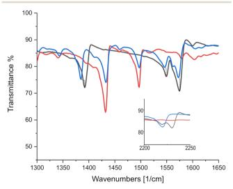
Fig. 7 IR absorption spectra identifying significant charge sensitive mode displacements between TCNQF<sub>2</sub> and triphenylene-TCNQF<sub>2</sub>. Black, red and blue lines represent TCNQF2, triphenylene and the triphenylene-TCNQF<sub>2</sub> co-crystal respectively. Inset displays C≡N markers at higher wavenumbers.
