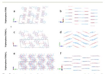
Fig. 3 Intermolecular displacements next to an expanded unit cell view down DA stack axis: triphenylene-TCNQ (a and b), triphenylene-TCNQF<sub>2</sub> (c and d) and triphenylene-TCNQF<sub>4</sub> (e and f). Triphenylene donor molecules are in blue, while  $TCNQF_n$  acceptor molecules are in red.
