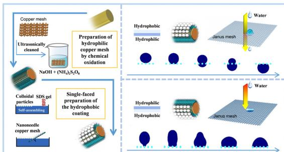
**Preparation of a Janus copper mesh *via* nanoparticle interface self-assembly for unidirectional water transportation**
