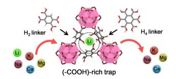
Constructing a carboxyl-rich angstrom-level trap in a metal-organic framework for the selective capture of lithium
