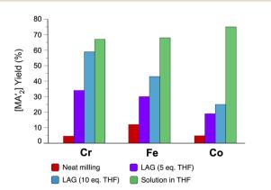
Fig. 8 Yields of  $[MA_2']$  complexes (M = Cr, Fe, Co) under conditions of neat milling, two regions of LAG, and in THF solution.<sup>23</sup>
