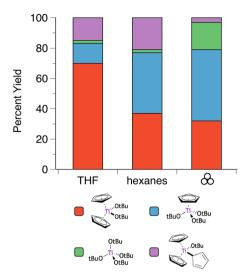
Fig. 5 Product selectivity for reactions of K[O<sup>t</sup>Bu] and Cp<sub>2</sub>TiCl<sub>2</sub> (2:1 molar ratio) under solution and mechanochemical conditions. 40
