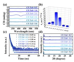
Fig. 3 (a) CD spectra, (b)  $g_{abs}$ -factor values at maximum CD peak, (c) TRPL spectra and (d) XRD patterns of 2D double (R-MPEA)<sub>4</sub>AgBiBr<sub>8</sub> perovskites synthesized at different volume ratios of chloroform (CF)/toluene (Tol).
