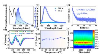
Fig. 2 (a) UV absorption and PL emission spectra of (R-MPEA)<sub>4</sub>AgBiBr<sub>8</sub> NBs. (b) Temperature-dependent PL spectra, (c) time-resolved PL decays spectra, (d) temperature-dependent CD spectra, (e) corresponding CD intensity at CD peaks of 420 nm and (f) PL intensity of (R-MPEA)<sub>4</sub>AgBiBr<sub>8</sub> NBs under ambient conditions with the relative humidity of RH = 65  $\pm$  5%.
