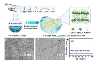
Fig. 1 (a) Schematic illustration of co-antisolvent modulation strategy via LARP for the synthesis, (b) SEM, (c) TEM images and (d) XRD pattern of the 2D double perovskite (R-MPEA)<sub>4</sub>AgBiBr<sub>8</sub> NBs.
