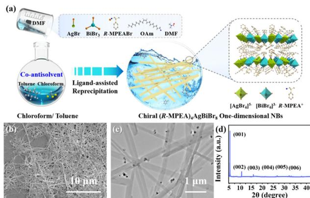
Fig. 1 (a) Schematic illustration of co-antisolvent modulation strategy via LARP for the synthesis, (b) SEM, (c) TEM images and (d) XRD pattern of the 2D double perovskite  $(R\text{-MPEA})_4\text{AgBiBr}_8$  NBs.
