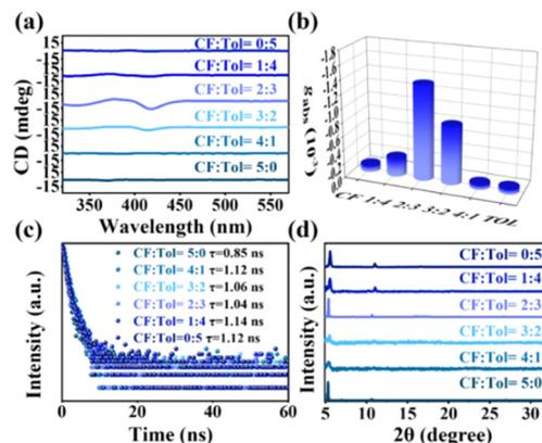
Fig. 3 (a) CD spectra, (b)  $g_{\text{abs}}$ -factor values at maximum CD peak, (c) TRPL spectra and (d) XRD patterns of 2D double  $(R\text{-MPEA})_4\text{AgBiBr}_8$  perovskites synthesized at different volume ratios of chloroform (CF)/toluene (Tol).
