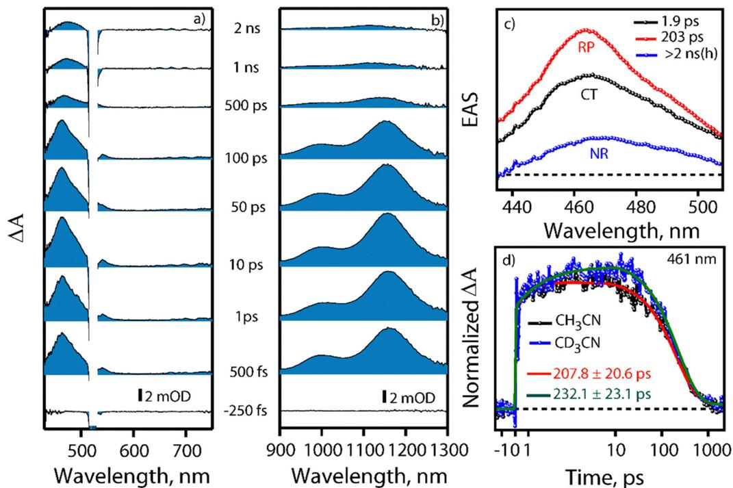
Fig. 3 Transient absorption (TA) data of 1-MePy c ExBox<sup>4+</sup> in CH<sub>3</sub>CN; (a) visible region and (b) NIR region. (c) SVD of TA data with 3-state sequential model: CT-Charge Transfer, RP: Radical Pair, NR: Neutral Radical state. (d) Normalized kinetics of TA data at 461 nm for the 1-MePy c ExBox<sup>4+</sup> complex in CH<sub>3</sub>CN and CD<sub>3</sub>CN.
