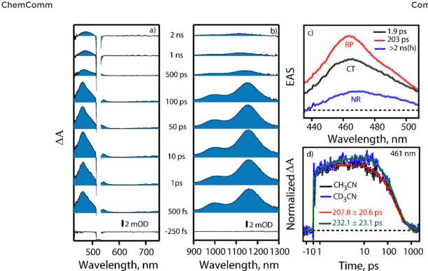
Fig. 3 Transient absorption (TA) data of 1-MePy  $\subset$  ExBox<sup>4+</sup> in CH<sub>3</sub>CN; (a) visible region and (b) NIR region. (c) SVD of TA data with 3-state sequential model: CT-Charge Transfer, RP: Radical Pair, NR: Neutral Radical state. (d) Normalized kinetics of TA data at 461 nm for the 1-MePy  $\subset$  ExBox<sup>4+</sup> complex in CH<sub>3</sub>CN and CD<sub>3</sub>CN.
