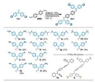
Scheme 1 Synthesis of N-benzidine benzophenone imines 2a-l including crystal structures of imines 2g and 2i.
