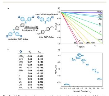
Fig. 2 (a) Reaction scheme of acid catalyzed imine hydrolysis, (b) kinetic plot  $ln(A/A_0)$  vs. t (linear regressions) following the hydrolysis of benzophenone imines at the absorption maximum in 1,4-dioxane, 50 °C, (c) reaction rate constants and para-Hammett parameters  $\sigma_p$  and (d) reaction rate constant  $k_{\rm obs}$  vs. Hammett parameter  $\sigma_{\rm p}$
