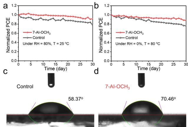
Fig. 4 Long-term stability of the inorganic CsPbBr<sub>3</sub> PSCs at (a) RH = 80%, T = 25 °C and (b) RH = 0%, T = 80 °C. The water contact angle of (c) control and (d) 7-AI-OCH<sub>3</sub>-based perovskite films.
