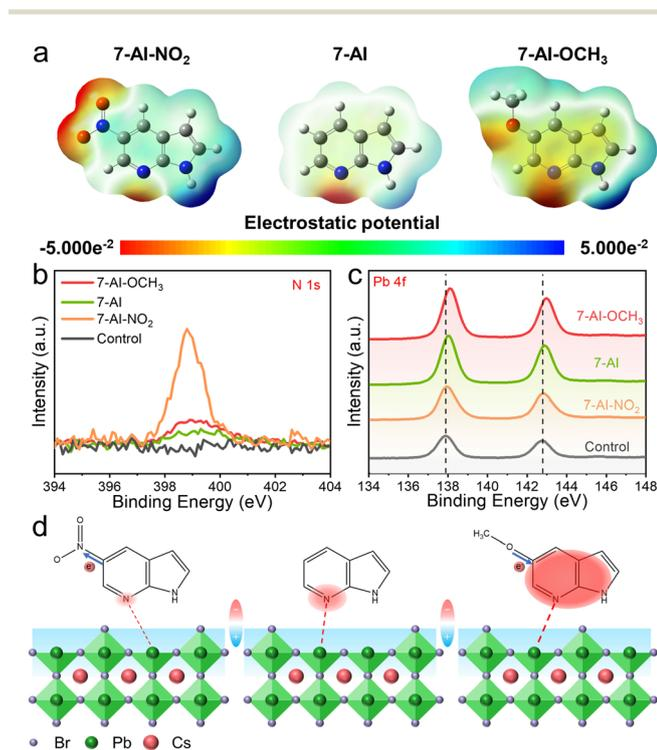
**Fig. 1** (a) Molecular structures and electrostatic potential maps of 5-nitro-7-azaindole (7-AI- $\text{NO}_2$ ), 7-azaindole (7-AI), and 5-methoxy-7-azaindole (7-AI- $\text{OCH}_3$ ). XPS spectra of (b) N 1s and (c) Pb 4f in  $\text{CsPbBr}_3$  films without and with organic molecule treatment. (d) Schematic diagram of electron-transfer-induced coulomb force regulation and the N atom passivated uncoordinated  $\text{Pb}^{2+}$ .
