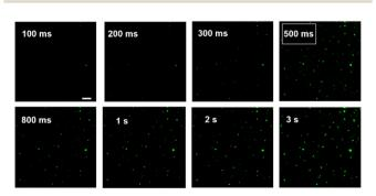
Fig. 3 ECL image of Co<sub>3</sub>O<sub>4</sub> at ITO slides with different exposure times; the applied potential was 1 V. Scale bar:  $5 \mu m$ .
