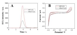
Fig. 1 (A) ECL profiles and (B) CV curves of the L012-H<sub>2</sub>O<sub>2</sub> system at the ITO surface with and without  $Co_3O_4$ . Working solution: 10 mM PBS containing 200  $\mu$ M L012. Scan range: -1.0 to 1.0 V, scan rate: 0.1 V s<sup>-1</sup>, PMT voltage: 600 V.
