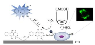
Scheme 1 ECL mechanism based on the Co<sub>3</sub>O<sub>4</sub> nanozyme for CEA antigen imaging at the cellular membrane.
