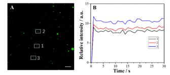
Fig. 4 (A) ECL image of  $Co_3O_4$  at ITO slides; (B) the fluctuation of ECL intensity at three particles labeled as 1, 2 and 3 in (A). The exposure time was 500 ms; the applied potential was 1 V. Scale bar: 5 μm.
