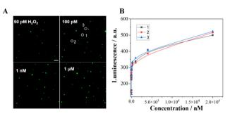
Fig. 5 (A) ECL image of Co<sub>3</sub>O<sub>4</sub> at ITO slides with different concentrations of H<sub>2</sub>O<sub>2</sub>; the exposure time was 500 ms, and the applied potential was 1 V. (B) Correlation between the luminescence of three particles and the concentration of H<sub>2</sub>O<sub>2</sub>. Scale bar: 5 μm.
