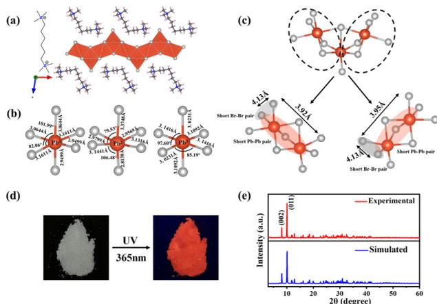
**Fig. 1** (a) Crystal structure of (HM)Pb<sub>2</sub>Br<sub>6</sub>. (b) The Pb–Br bond lengths and Br–Pb–Br bond angles of three individual polyhedra. (c) The detailed view of the Pb–Pb and Br–Br pair distance determined from the SCXRD analysis. (d) Photographs of (HM)Pb<sub>2</sub>Br<sub>6</sub> single crystals under ambient light (left) and UV 365 nm light (right). (e) The experimental and simulated XRD patterns of (HM)Pb<sub>2</sub>Br<sub>6</sub>.
