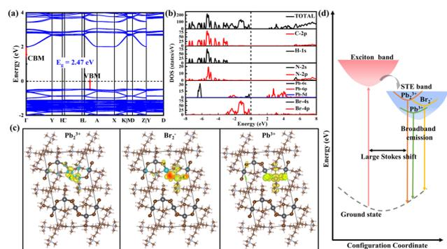
Fig. 4 (a) Calculated electronic band structures and (b) DOS of (HM)Pb<sub>2</sub>Br<sub>6</sub>. (c) Calculated charge density for (HM)Pb<sub>2</sub>Br<sub>6</sub> (Pb<sub>2</sub><sup>3+</sup>, Br<sub>2</sub><sup>-</sup> and Pb<sub>3</sub><sup>+</sup> STLHs holes) upon crystal lattice perturbation via the Pb–Pb, Br–Br and Pb–Br distances shortening. (d) Configuration coordinate diagram illustrating the luminescence mechanism.
