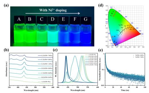
Fig. 1 (a) Images under UV-light (365 nm), (b) UV-vis absorption spectra, (c) PL spectra, and (d) CIE coordinates for  $Ni^{2+}$  doped FAPbBr<sub>3</sub> QDs. (e) PL decay curves of deep blue QD solutions with Ni/Pb ratios of 4.86% and 7.96% (measured emission wavelength: 442 nm).
