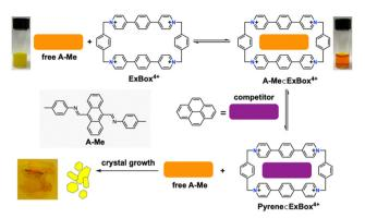
Fig. 2 Host-mediated single crystal growth of an anthracene bisimine guest A-Me. As a competitor guest (pyrene) diffuses in slowly, A-Me is released from ExBox<sup>4+</sup> and rapidly begins crystalizing. Further growth of crystals is sustained by the continuous dissociation of the host-quest complex and the release of the guest A-Me from ExBox<sup>4+</sup> host.
