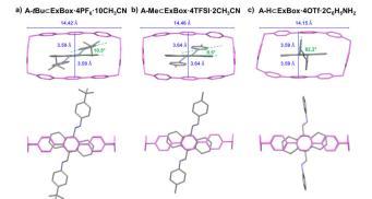
Fig. 4 Crystal structures of host-guest complexes of A-R in ExBox<sup>4+</sup>. All crystals were grown by vapor diffusion of iPr<sub>2</sub>O into the solutions containing A-R⊂ExBox·4X complexes in MeCN. Hydrogens, counterions, solvent molecules, and interstitial aniline in the case of A-H = ExBox-4OTf-2C<sub>6</sub>H<sub>5</sub>NH<sub>2</sub>, are omitted for clarity.
