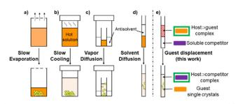
Fig. 1 Various methods used to grow single crystals from solution. (a) Slow evaporation of solvent, (b) slow cooling of a hot solution, (c) vapor diffusion of an antisolvent using a saturated solution of the analyte, (d) diffusion of an antisolvent layered on top of the analyte solution, and (e) displacement of the guest encapsulated in a soluble macrocyclic host by a competitor (this work)
