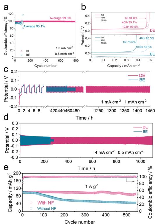
**Fig. 4** (a) Coulombic efficiencies of Zn||Cu cells at  $1 \text{ mA cm}^{-2}$  and corresponding (b) charge/discharge curves. Cycling performances of Zn||Zn cells at (c)  $1 \text{ mA cm}^{-2}$  and  $1 \text{ mA h cm}^{-2}$ , and (d)  $4 \text{ mA cm}^{-2}$  and  $0.5 \text{ mA h cm}^{-2}$ . (e) Cycling capabilities of Zn|| $\text{MnO}_2$  cells at  $1 \text{ A g}^{-1}$ .
