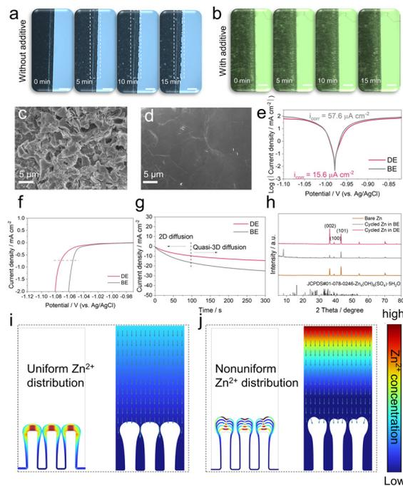
**Fig. 2** *In situ* optical microscopy images of Zn||Zn cells at 10 mA cm<sup>-2</sup> in (a) BE and (b) DE (scale bar: 300 μm). SEM images of cycled zinc foils in (c) BE and (d) DE. (e) Linear polarization curves of zinc anodes. (f) HER performances. (g) CA curves of Zn plates at -150 mV. (h) XRD patterns of the bare Zn and cycled Zn. COMSOL simulation results of the zinc concentrations of the (i) DE system and (j) BE system.
