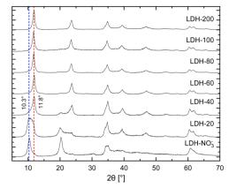
Fig. 1 PXRD patterns of pristine LDH- $NO_3$  and the anion exchanged samples LDH-A (A = 20, 40, 60, 80, 100 and 200 standing for the initial carbonate concentration in mmol  $L^{-1}$  in the anion exchange solution). The NO<sub>3</sub><sup>-</sup>- and CO<sub>3</sub><sup>2-</sup>-intercalated phases can be identified by the characteristic basal reflections at 10.3 and 11.8°  $2\theta$ , respectively
