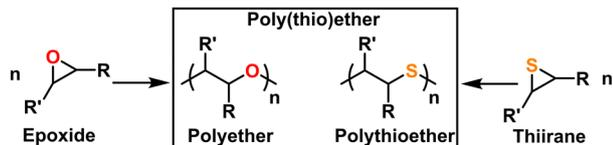
Fig. 1 Common monomers and polymer structures for poly(thio)ethers.
