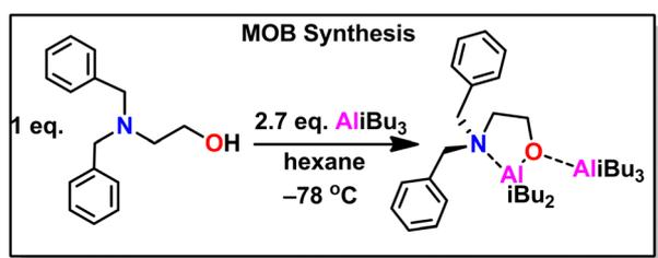
Fig. 30 Synthesis of the MOB catalyst/initiator for epoxide polymerizations.
