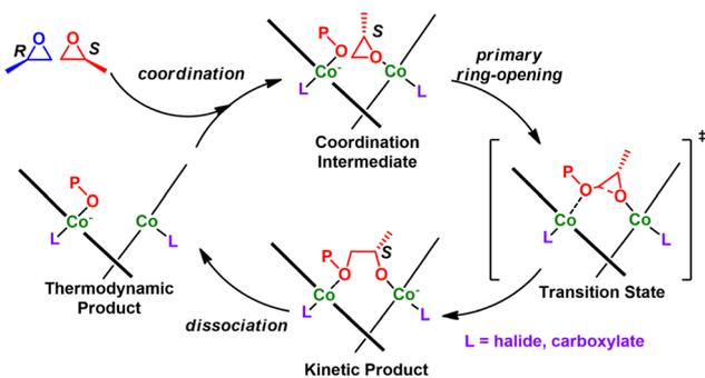
Fig. 26 Enantioselective polymerization with double cobalt catalyst.
