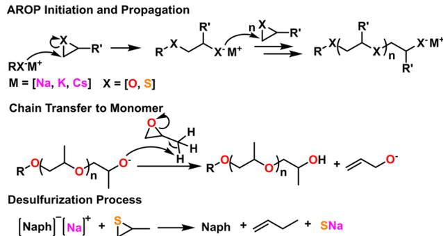
Fig. 5 (Top) General AROP initiation and propagation mechanism. (middle) Chain transfer to monomer, a common side reaction with epoxides. (Bottom) Desulfurization process endemic to thiirane AROP.
