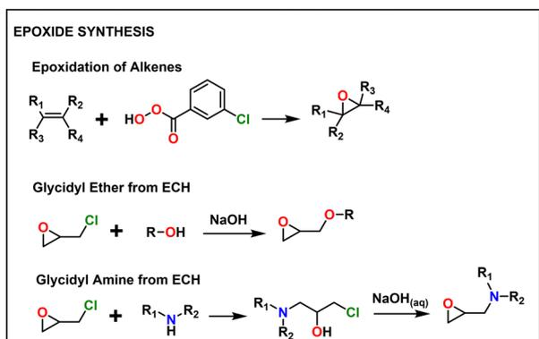
Fig. 2 Common epoxide synthesis methods.
