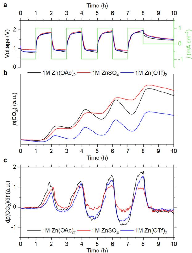
Fig. 1 Cell voltage and current density vs. time (a), evolution of the CO<sub>2</sub> partial pressure (b) and its derivative (c) during the OEMS measurements with 1 M electrolytes.
