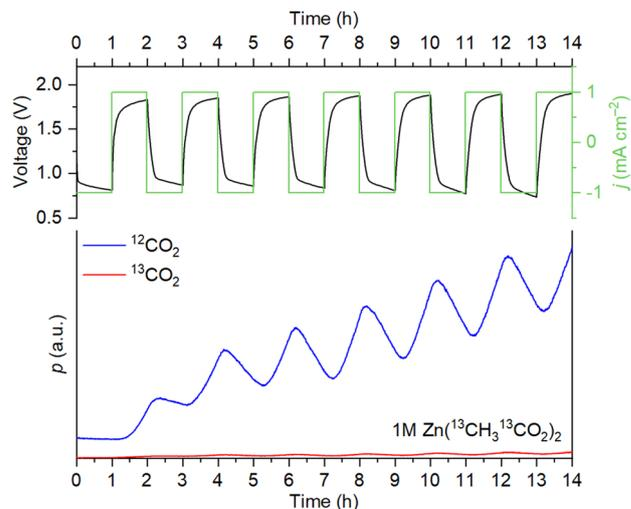
Fig. 2 Cell voltage/current density vs. time and evolution of <sup>12</sup>CO<sub>2</sub>/<sup>13</sup>CO<sub>2</sub> during the OEMS measurements with 1 M Zn(<sup>13</sup>CH<sub>3</sub><sup>13</sup>CO<sub>2</sub>)<sub>2</sub> as the electrolyte.
