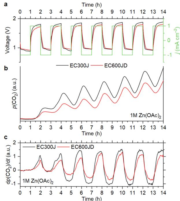
Fig. 4 Cell voltage and current density vs. time (a), evolution of  $\text{CO}_2$  partial pressure (b) and its derivative (c) during the OEMS measurements with different types of carbon black. The electrolyte was  $1 \text{ M Zn}(\text{OAc})_2$ .
