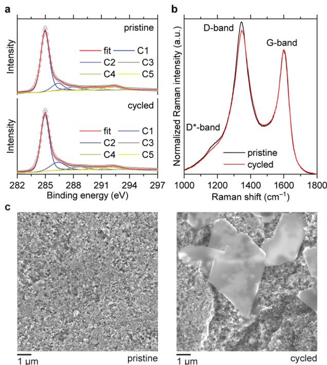
Fig. 3 XPS (a), Raman spectra (b) and SEM images (c) of the carbon electrodes before and after 10 cycles at  $1 \text{ mA cm}^{-2}$  with a fixed capacity of  $1 \text{ mA h cm}^{-2}$ . The electrolyte was  $1 \text{ M ZnSO}_4$ .
