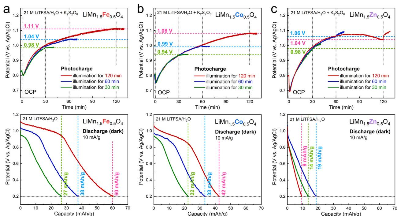
Fig. 3 (a)–(c) Open circuit potential (OCP) during the photocharging process under illumination in 21 M LiTfSA/ $\text{H}_2\text{O}$  with  $\text{K}_2\text{S}_2\text{O}_8$  as an electron acceptor (upper) and discharging profiles in the dark condition for the electrodes after photocharging (lower), where the electrolyte used in the discharging process was 21 M LiTfSA/ $\text{H}_2\text{O}$  without  $\text{K}_2\text{S}_2\text{O}_8$ .
