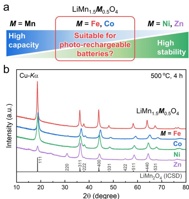
Fig. 2 (a) Overview of the materials design strategy in this study. (b) XRD profiles of the synthesized  $\text{LiMn}_{1.5}\text{M}_{0.5}\text{O}_4$  (M = Fe, Co, Ni, Zn) after calcination at 500 °C for 4 h.
