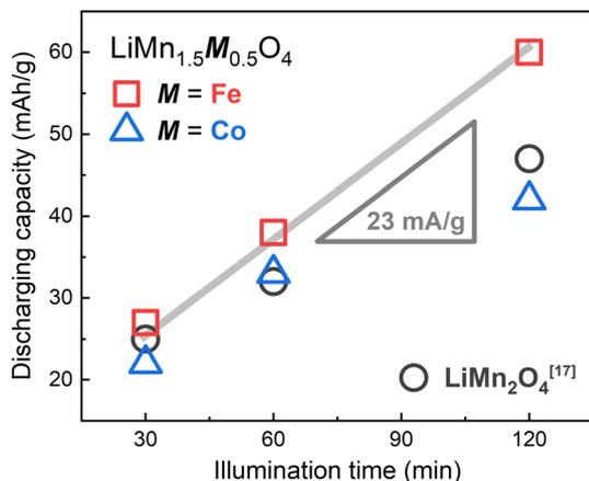
Fig. 4 Discharge capacities of  $\text{LiMn}_{1.5}\text{M}_{0.5}\text{O}_4$  ( $\text{M} = \text{Fe}, \text{Co}$ ) after the photocharging process together with our previous data for  $\text{LiMn}_2\text{O}_4$ .<sup>17</sup> The grey line indicates the previously estimated photocharging rate in our photoelectrochemical system with  $\text{TiO}_2$  and  $\text{K}_2\text{S}_2\text{O}_8$ .<sup>17</sup>
