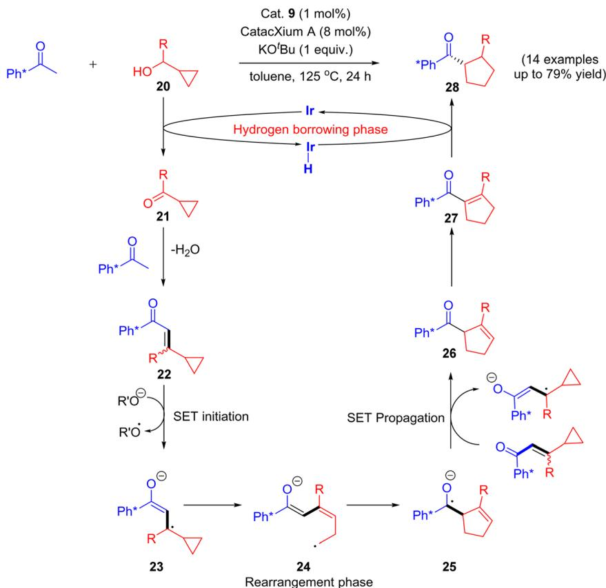
Scheme 12 Iridium-catalyzed hydrogen borrowing cascade reaction via a vinyl cyclopropane ring expansion.
