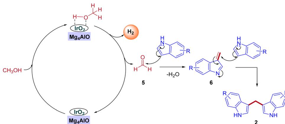
**Scheme 6** Plausible reaction mechanism for the coupling of indoles with methanol under heterogeneous iridium catalysis.
