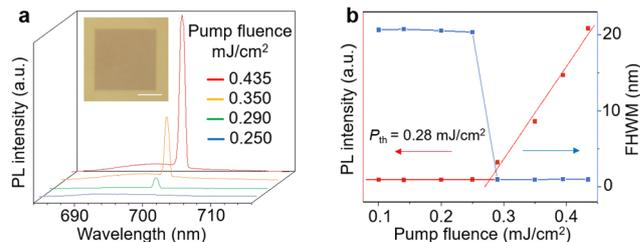
Fig. 3 (a) PL spectra of the BIPS@PMMA film-covered Ag nanoparticle array at different pump fluences. Inset: Bright-field microscopy image of the fabricated device. Scale bar is 50  $\mu\text{m}$ . (b) Emission intensity (red) and FWHM (blue) as a function of pump fluence.
