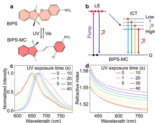
**Fig. 1** (a) Reversible photoisomerization of BIPS between spiropyran and merocyanine forms. (b) Energy diagram for the concentration-dependent ICT process of BIPS-MC. (c) PL spectra from a 20 wt% BIPS@PMMA film at different UV exposure times. (d) Refractive indices of the BIPS@PMMA film with increasing exposure time to UV light.
