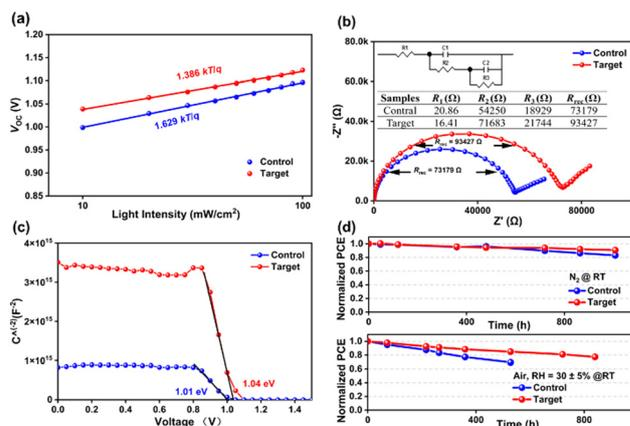
Fig. 4 (a)  $V_{oc}$  vs. light intensity, (b) EIS and (c) Mott–Schottky fitting to the capacitance–voltage plots for the control and target devices. (d) Stability of unencapsulated devices under  $N_2$  and air conditions.
