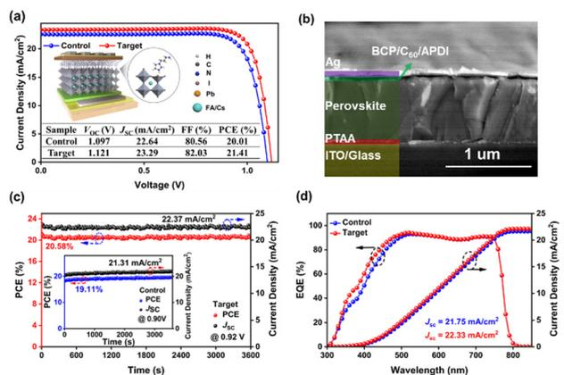
Fig. 3 (a)  $J$ - $V$  curve of PSCs and the illustration of device structure based on APDI modification, (b) cross-sectional SEM image of PSC, (c) stabilized power output at the maximum power point under AM 1.5G and (d) EQE for the control and target devices.
