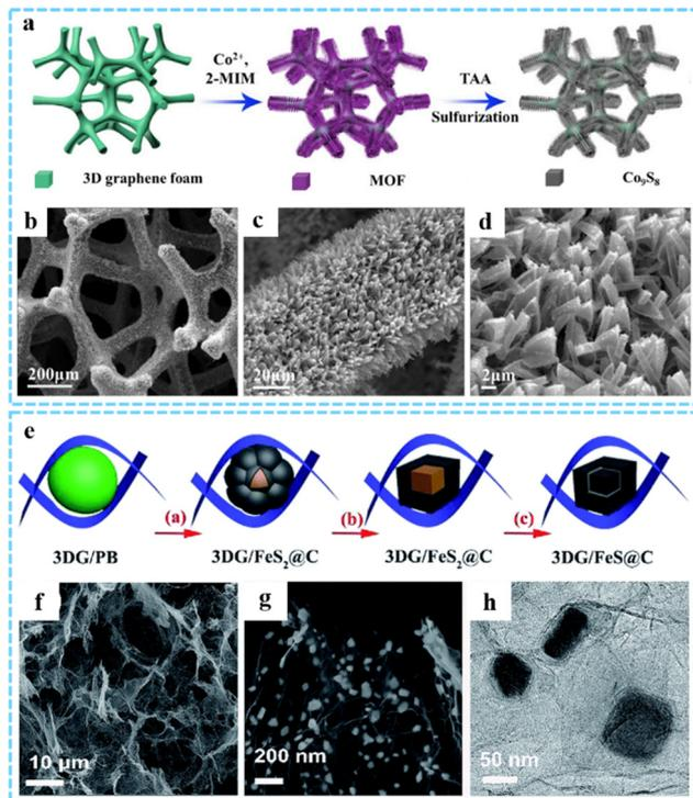
Fig. 6 (a) Schematic illustration of the synthetic route of the Co<sub>9</sub>S<sub>8</sub>-3DGf composites. (b)–(d) SEM images of Co<sub>9</sub>S<sub>8</sub>-3DGf. Reprinted with permission from ref. 94. Copyright 2018 Elsevier. (e) Illustration of the synthesis process of the 3DG/FeS@C composites. (f) and (g) SEM and (h) TEM of DG/FeS@C. Reproduced with permission from ref. 81. Copyright 2018 Royal Society of Chemistry.
