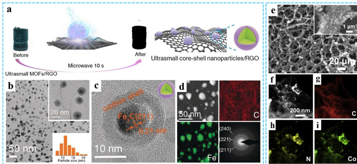
**Fig. 8** (a) Schematic illustration of the fabrication process of  $\text{Fe}_3\text{C}@C/\text{RGO}$ . (b) TEM and (c) HRTEM images of  $\text{Fe}_3\text{C}@C/\text{RGO}$ . (d) STEM image, element mapping and SAED pattern. Reproduced with permission from ref. 78 Copyright 2020 Wiley-VCH. (e) SEM image of  $\text{CoN}_x/\text{NGA}$ . (f) HAADF and (g)–(i) EDXS images of  $\text{CoN}_x/\text{NGA}$ . Reprinted with permission from ref. 52. Copyright 2019 Elsevier.
