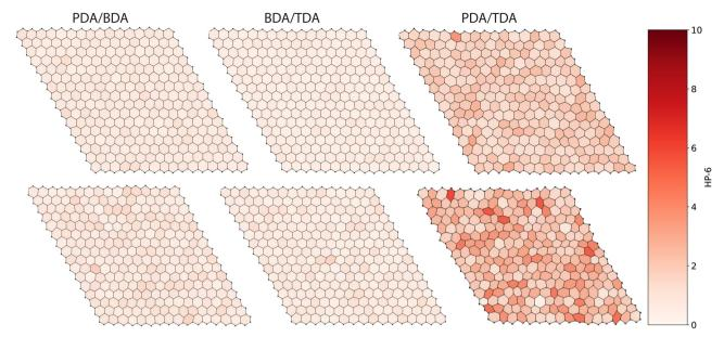
Fig. 5 Outlines of representative COF structures produced from the MC simulations with a correlated distribution of linkers (top) and randomly distributed linkers (bottom) for each linker combination. Hexagons within the structure are coloured by their similarity to a perfect hexagon, HP-6.
