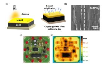
Fig. 6 Spray coating method. (a) The schematic diagram of spray coating. (b) Cross sectional SEM image of the MAPbI<sub>3</sub> film by spray coating. Reproduced with permission. 104 Copyright 2021, Elsevier. (c) Photograph of a circuit. (d) X-ray imaging of the circuit by the 2D (PEA)<sub>2</sub>MA<sub>3</sub>Pb<sub>4</sub>I<sub>13</sub>/3D MAPbl<sub>3</sub> detector.<sup>56</sup>
