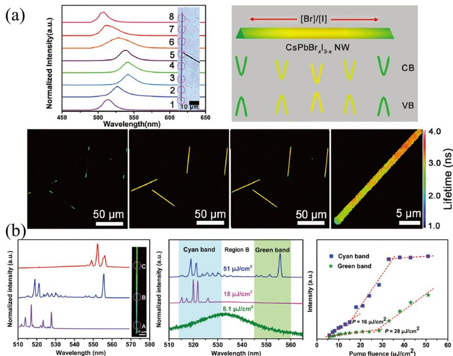
Fig. 13 (a) Position-dependent PL spectra, schematic diagram of the energy band level, confocal laser scanning microscope image and fluorescence lifetime imaging microscope images of CsPbBr<sub>x</sub>I<sub>3-x</sub> NW. (b) Characterization of the dual-color lasing in the compositional gradient CsPbBr<sub>x</sub>I<sub>3-x</sub> NW. (a) and (b) Reprinted with permission from ref. 89, Copyright 2018, John Wiley and Sons.
