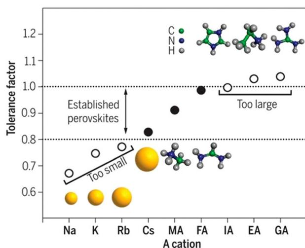
Fig. 1 Tolerance factor in HPs of ABX<sub>3</sub> structure. Reprinted with permission from ref. 26, Copyright 2019, American Chemical Society.
