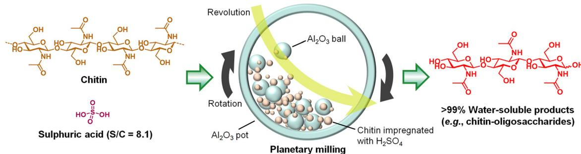
Fig. 5 Hydrolysis of chitin by  $\text{H}_2\text{SO}_4$  in the mechanochemical method.
