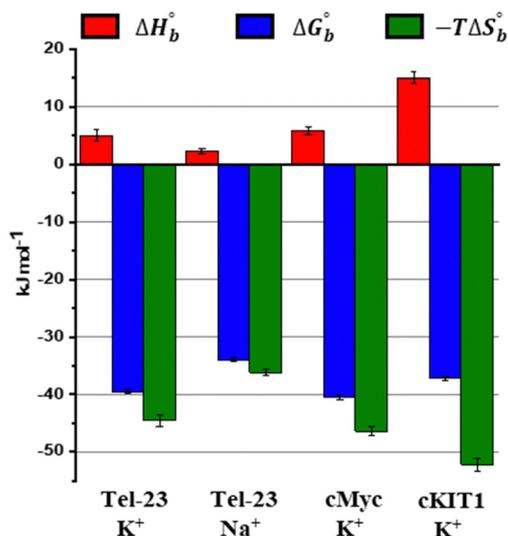
Fig. 3 Thermodynamic profiles for LL-III binding to the DNA G-quadruplexes. The sum of the binding enthalpy,  $\Delta H_b^\circ$ , (red) and the binding entropy multiplied by the absolute temperature,  $-T\Delta S_b^\circ$ , (green) provides the binding Gibbs energy,  $\Delta G_b^\circ$  (blue). All the thermodynamic parameters are given at 20 °C ( $T = 293$  K).
