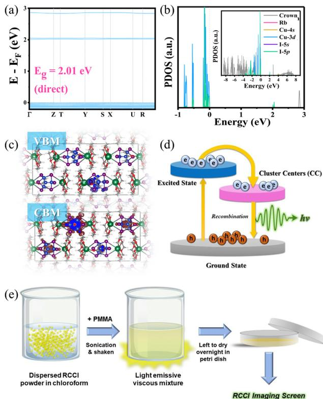
**Fig. 2** (a) Electronic band gap structure. (b) PDOS of RCCl; the inset shows a PDOS with a larger range. (c) Plots of wavefunction  $|\Psi|^2$  of the CBM and VBM. (d) Schematic diagram of the photophysical processes. (e) Schematic illustration of the preparation procedure of RCCl@PMMA imaging screens.
