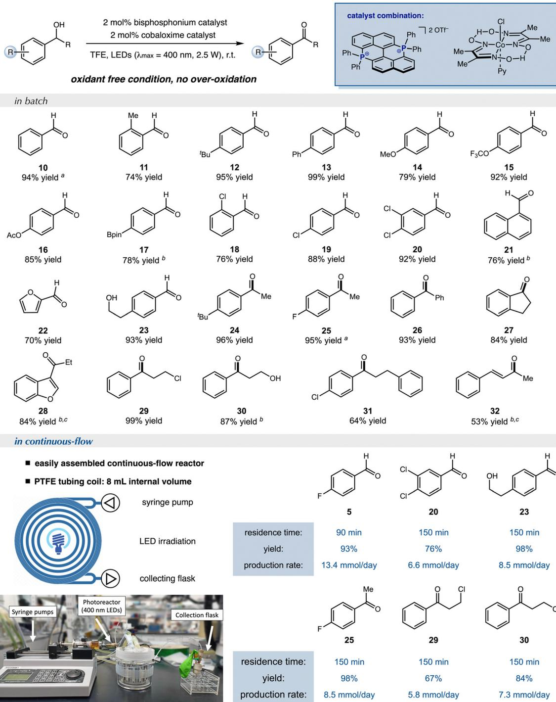
Fig. 3 Reaction scope. Batch reactions were performed at the 0.2 mmol scale, and isolated yields are shown. <sup>a</sup>Yields were determined via GC-FID due to volatile products. <sup>b</sup>4 mol% bisphosphonium **3** and 4 mol% cobaloxime were used. <sup>c</sup>MeCN was used instead of TFE. See ESI† for experimental details.
