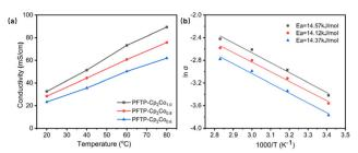
Fig. 1 (a)  $OH^-$  conductivity of PFTP- $Cp_2Co_x$  membranes at varied temperatures. (b) Arrhenius plots of hydroxide conductivity for the PFTP- $Cp_2Co_x$  membranes.
