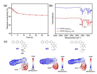
Fig. 2 (a) OH $^-$  conductivity variation of the PFTP-Cp<sub>2</sub>Co<sub>0.8</sub> membrane in 1 M KOH at 80  $^\circ$ C for 30 days. (b) FT-IR spectra of the PFTP-Cp<sub>2</sub>Co<sub>0.8</sub> membrane before and after alkaline treatment (PFTP-Cp<sub>2</sub>Co<sub>0.8</sub>: without alkali treatment; PFTP-Cp<sub>2</sub>Co<sub>0.8</sub>-OH $^-$ : treated in 1 M KOH at 80  $^\circ$ C for 30 days). (c) ESP of cobaltocenium M1, quaternary ammonium M2, and piperidinium M3.
