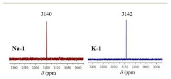
Fig. 3  $^{195}$ Pt NMR spectra of **Na-1** and **K-1** dissolved in H<sub>2</sub>O/D<sub>2</sub>O.
