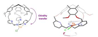
Fig. 11 Schematic representation of the chirality transfer observed in M-Cu<sup>I</sup>(Hm-CH<sub>2</sub>-TPA)(Cl) (left), along with view of its XRD structure (right).
