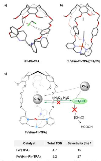
Fig. 9 Representation of the XRD structures of (a) Hm-Ph-TPA and (b) Cu<sup>II</sup>(Hm-Ph-TPA). (c) Concept of the selective methane to methanol oxidation via H<sub>2</sub>O<sub>2</sub> activation in Fe<sup>II</sup>(Hm-Ph-TPA), in water along with the comparison table between the open Fe(TPA) and the caged catalysts. <sup>a</sup> Selectivity toward primary oxidation products CH<sub>3</sub>OH and CH<sub>3</sub>OOH.
