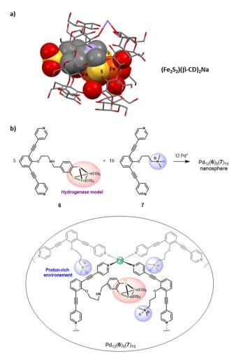
Fig. 7 (a) Representation of the XRD structure of (Fe<sub>2</sub>S<sub>2</sub>)(β-CD)<sub>2</sub>Na. (b) Confinement of five hydrogenase mimicking clusters in a proton reach the Pd<sub>12</sub>(6)<sub>5</sub>(7)<sub>19</sub> nanosphere (top), along with the schematic representation of one of the five catalytic centers found in the nanosphere (bottom).
