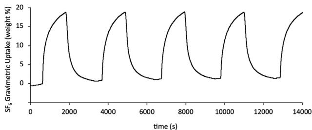
Fig. 4 TGA cyclic SF<sub>6</sub> uptake on **CTH-18**. Adsorption was carried out at 30 °C over 20 minutes, regeneration by heat (desorption) was carried out at 100 °C for 20 minutes.
