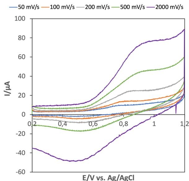
Fig. 6 Cyclic voltammetry at different sweep rates, see legends in phosphate buffer pH = 7. The electrode consisted of carbon paste and [Mn<sub>3</sub>(cpb)(dmf)<sub>3</sub>], **CTH-18**.
