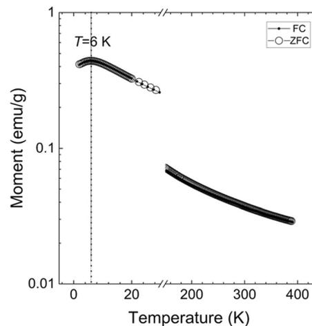
Fig. 5 Temperature dependence of the magnetization for **CTH-18**. An applied field of 1 kOe was used. Below the Néel transition at 6 K we can see the magnetic moment decrease as a result of the antiferromagnetic coupling and above 6 K we see paramagnetic behavior.
