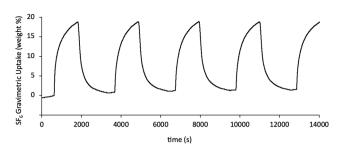
Fig. 4 TGA cyclic SF $_6$  uptake on **CTH-18**. Adsorption was carried out at 30  $^{\circ}$ C over 20 minutes, regeneration by heat (desorption) was carried out at 100  $^{\circ}$ C for 20 minutes.
