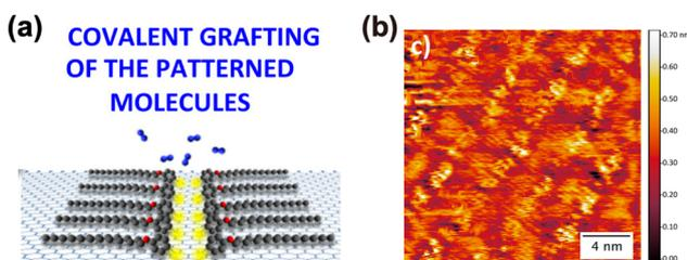
**Fig. 12** (a) Scheme of the covalent grafting of patterned molecules on the surface of graphene. (b) STM height image of molecules self-assembled on graphene. Reproduced with permission.<sup>46</sup> Copyright 2016, American Chemical Society.
