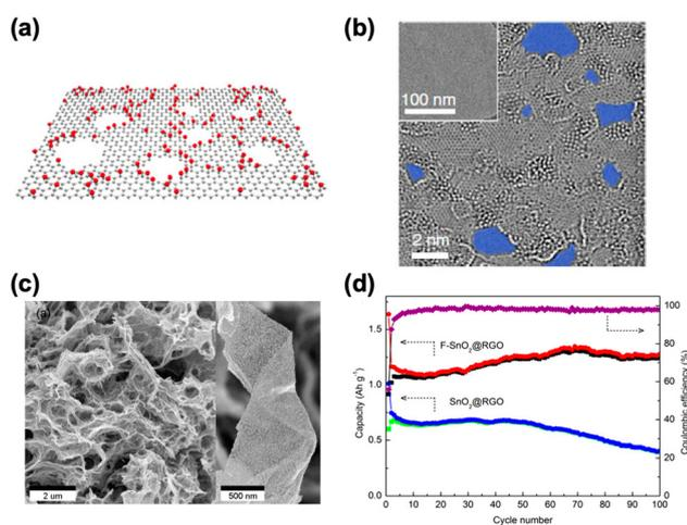
**Fig. 5** (a) Schematic models of porous GO. (b) An HR-TEM image of GO sheets. Reproduced with permission.<sup>25</sup> Copyright 2019, Springer Nature. (c) SEM image of F-SnO<sub>2</sub>@RGO composite. (d) Cycling stabilities of the F-SnO<sub>2</sub>@RGO and SnO<sub>2</sub>@RGO electrodes and the corresponding Coulombic efficiency. Reproduced with permission.<sup>26</sup> Copyright 2015, American Chemical Society.
