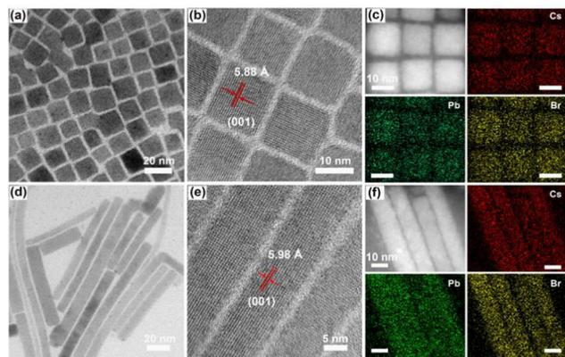
**Fig. 1** (a) TEM image, (b) high-resolution TEM image and (c) corresponding elemental mapping of Cs, Pb and Br elements, respectively, over 3D NCs. (d) TEM image, (e) high-resolution TEM image and (f) corresponding elemental mapping of Cs, Pb and Br elements, respectively, over 1D NRs.
