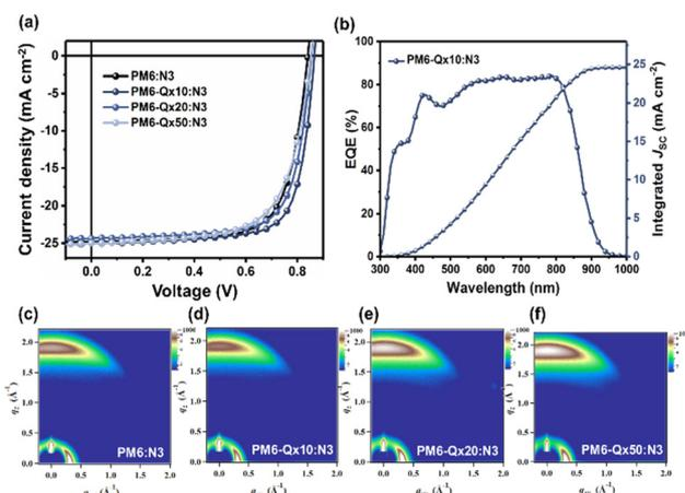
Fig. 2 (a)  $J$ - $V$  curves of the fabricated OSCs based on the polymer donor:N3 blends. (b) Corresponding EQE spectra of the optimized device based on PM6-Qx10:N3. (c–f) 2D GIWAX images of PM6- and PM6-Qx-based blend films.
