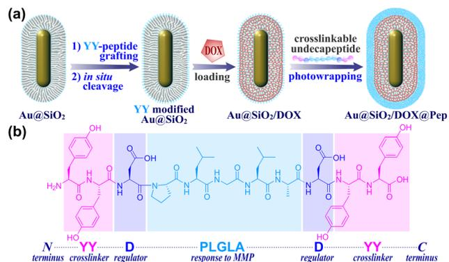
**Scheme 1** (a) The fabrication of peptide-photowrapped Au@SiO<sub>2</sub>/DOX@Pep nanocapsules, and (b) the design of crosslinkable undecapeptide.
