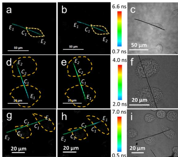
**Fig. 3** The FLIM images of the NWFLT incubated with a single cell at different temperatures (a) 27.0 °C and (b) 38.0 °C. (c), (f) and (i) are the DIC images. The FLIM images of the NWFLT with (d) and without (e) 10 mM  $\text{Ca}^{2+}$ , and the FLIM images of the NWFLT with (g) and without (h) 10  $\mu\text{M}$  CCCP, and the cells are noted by the yellow dotted line. The endpoints of the NWFLT are marked as point E, and the contact positions of the cell membrane with NWFLT are marked as C.
