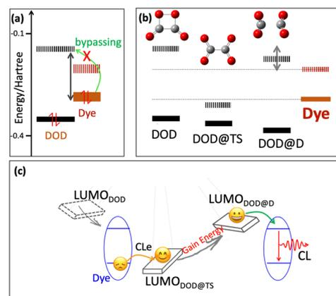
**Fig. 3** Electronic properties of the CL system. (a) The relative HOMO and LUMO energy levels of the DOD and cyanine dyes. (b) The relative HOMO and LUMO energy levels of the DOD, DOD@TS (Transition State), DOD@D (Dissociated state) and cyanine dyes. (c) Orbital swing scheme for the electron transfer of the single-dye NIR-II CL system.
