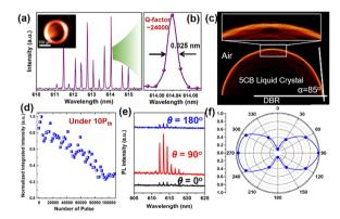
Fig. 2 (a) Typical lasing spectrum from an LC-DSM microlaser with a diameter of 190  $\mu m$ . (b) The FWHM and Q-factor of a single lasing peak. (c) The simulated distribution of electric field in the LC-DSM microcavity. (d) The stability of the LC-DSM microlaser. (e) Lasing spectra from the same monolithic microlaser under various rotation angles ( $\theta$ ) of the linear polarizer. (f) Normalized intensity of lasing as a function of various  $\theta$ .
