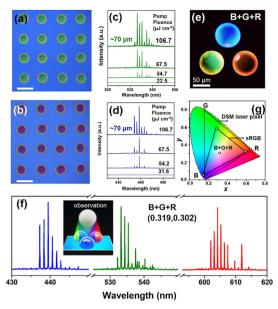
Fig. 3 (a)-(d) Bright-field images and power-dependent PL spectra of LC-DSM microlaser arrays in the green and blue emission bands. Scale bar 50 μm. (e) Photoluminescence images of a single display pixel cell consisting of a set of adjacent RGB LC-DSM microlasers. (f) Full-color lasing from the pixel array. (g) Comparison of the color gamut between an individual printed RGB pixel and the standard color space.
