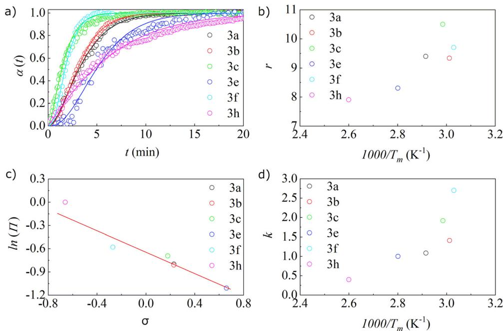
Fig. 2 (a) Global molar fraction  $\alpha(t)$  as a function of milling time ( $t$ ), (b) interface generation rate  $r$  as a function of reciprocal of temperature, (c) semi-logarithmic plot of reaction probability at interface as a function of Hammett substituent constants, and (d) volume fraction of powder undergoing CLCs as a function of reciprocal of temperature.
