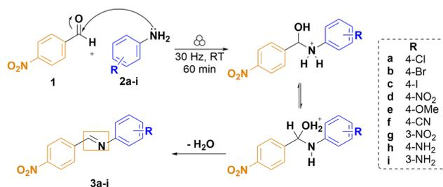
Scheme 1 Neat grinding reaction of imine formation from (**1**) and substituted anilines (**2a–i**) and the proposed reaction mechanism in solution.<sup>16</sup>
