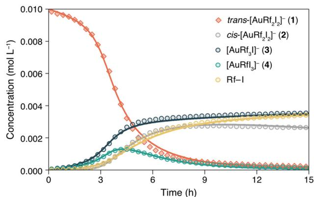
Fig. 2 Concentration vs. time plot of experimental data (dots) obtained by  $^{19}\text{F}$  NMR monitoring and COPASI-fitted values (continuous lines) of the fluorinated-species observed when heating complex **1** in TCE- $d_2$  at 338 K.
