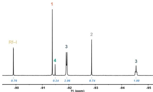
Fig. 1  $F_{ortho}$  region of the  $^{19}\text{F}$  NMR spectrum recorded from solutions of **1** in TCE- $d_2$  after heating at 323 K for 1 day. Assignment of the signals and corresponding integrals.
