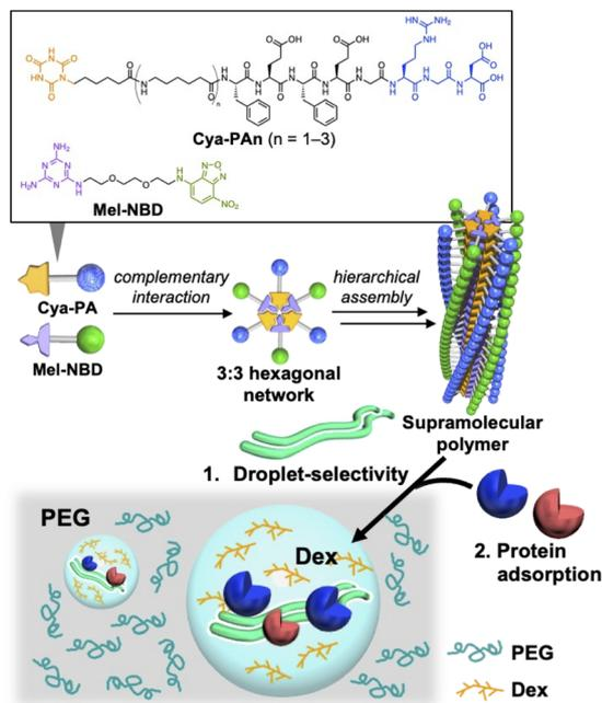
**Fig. 1** Chemical structures of Cya-PA and Mel-NBD, and a schematic representation of this study. A supramolecular polymer formed by complementary interaction and hierarchical assembly shows droplet-selectivity in the PEG/Dex liquid-liquid phase separation. Proteins adsorbed on the supramolecule are recruited to the droplets.
