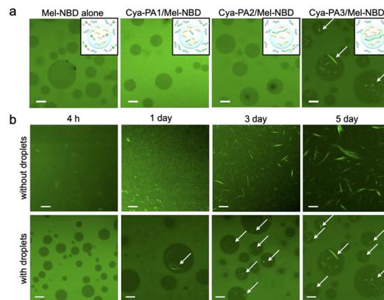
**Fig. 2** (a) Phase selectivity of Mel-NBD alone and co-assemblies with Cya-PA. Mel-NBD alone, Cya-PA1/Mel-NBD, and Cya-PA2/Mel-NBD show relatively high accumulation in the PEG phase, while bundled fibers of Cya-PA3/Mel-NBD are localized in Dex droplets. (b) Time-dependent co-assembly formation with or without LLPS droplets formed using 5 wt% PEG and Dex. [Cya-PA/Mel-NBD] = 1.5 mM. Bars: 10  $\mu$ m. White arrows denote Cya-PA3/Mel-NBD fibers in Dex droplets.
