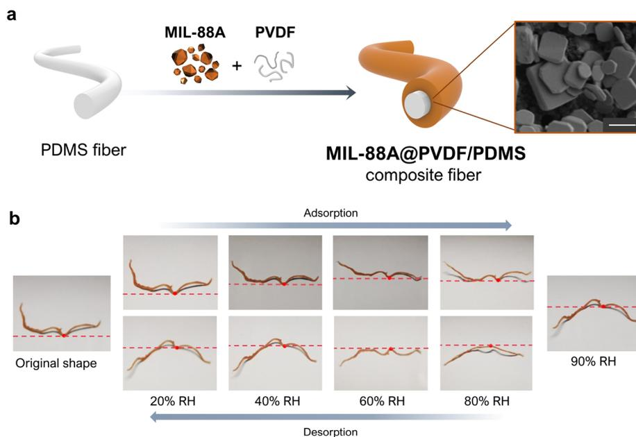
**Fig. 6** (a) Schematic of the fabrication of the MIL-88A@PVDF/PDMS fibres (left). SEM image of a MIL-88A@PVDF/PDMS fibre, revealing the embedding of MIL-88A within the PVDF polymer matrix (right). Scale bar (1  $\mu\text{m}$ ). (b) Photographs of the deformation of MIL-88A@PVDF/PDMS fibre upon exposure to different levels of relative humidity (RH): from 20% up to 90% (adsorption), and from 90% back down to 20% (desorption). Adapted, with permission, from ref. 54.
