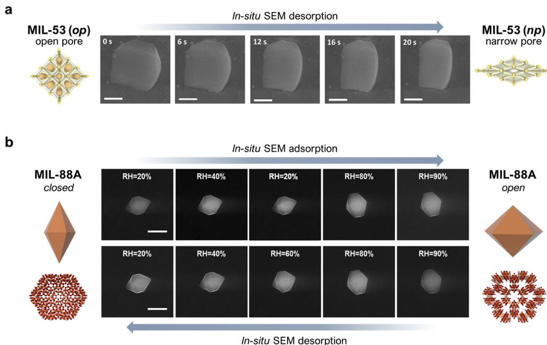
**Fig. 1** (a) *In situ* FESEM images showing variations in the single-crystal dimensions of MIL-53(Al) over time. Scale bars = 500 nm. (b) *In situ*, humidity-controlled FESEM images of a single crystal of MIL-88A at different levels of relative humidity (RH). Top row: adsorption (from 20% RH up to 90% RH); Bottom row: desorption (from 90% RH back down to 20% RH). Scale bar = 5  $\mu$ m. Adapted, with permission, from ref. 29 and 30.
