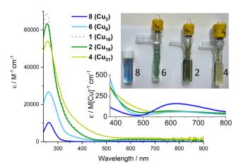
Fig. 4 UV/vis spectra of 2, 4, 6 & 8 reported as molar extinction coefficients. Spectra recorded at 0.1-0.4 mM[Cu] in CH2Cl2 (or pentane for 2), inset shows magnified visible region as 'per copper' normalised extinction coefficients, spectra recorded at 1.7-3.3 mM[Cu]). Photos of solutions (with  $[Cu] = \sim 0.24 \text{ mM}$ ).
