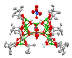
Fig. 3 Solid-state structure of 7. Ellipsoids displayed at 50% probability, hydrogen atoms (except OH groups) and [NEt<sub>3</sub>H]<sup>+</sup> cations omitted for clarity. Cu = green, O = red, C = grey, N = blue, H = very pale blue. The base of the structure (within the pocket) has disordered O'Pr and OH groups
