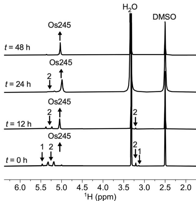
Fig. 1  $^1\text{H}$  NMR spectra (500 MHz, 25 °C,  $\text{DMSO}-d_6$ ) showing the conversion of **1** and **2** to Os245 by heating in refluxing HCl. Arrows indicate the growth or disappearance of peaks.
