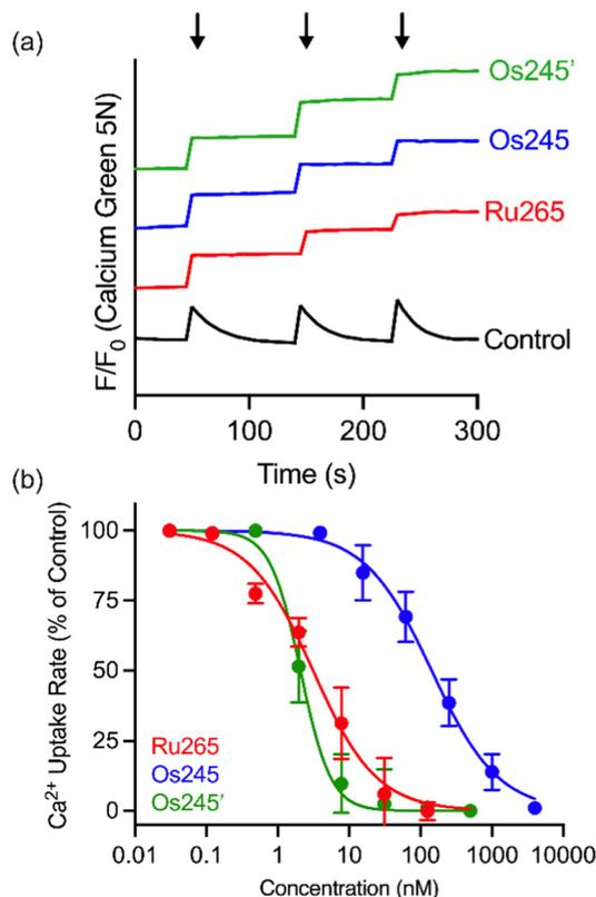
Fig. 3 (a) Representative traces of extramitochondrial Ca<sup>2+</sup> clearance in permeabilized HeLa cells ( $5 \times 10^6$  cells mL<sup>-1</sup>) treated with 1 μM of Ru265, Os245 or Os245'. Arrows indicate addition of 10 μM Ca<sup>2+</sup>. The traces are vertically offset for clarity. (b) Dose-response curve for mt-Ca<sup>2+</sup> uptake inhibition by Ru265, Os245, and Os245' in permeabilized HeLa cells. Data are represented as the mean ± SD ( $n = 4–5$ ).
